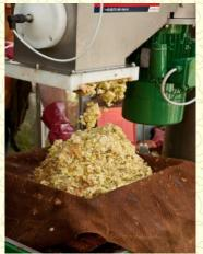
It takes around 100 kg of apples to make a cheese for our Voran hydraulic press - the cheese is built up using nine layers of pomace wrapped in pressing cloths and separated by ten wooden racks. Once built, the cheese is moved across the press so pressing can begin.
